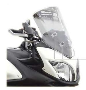
REMOVE THE 4 ORIGINAL FIX SCREWS AND ORIGINAL THICKNESS
