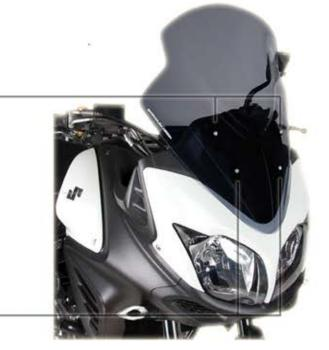
INSTALL THE WINDSHIELD/SCREEN USING THE SPECIFIC ALUMINUM THICKNESS AND RUBBER AND TEFLON WASHERS INCLUDED IN THE BARRACUDA INSTALLATION KIT. PUT THE TEFLON WASHERS UNDER THE HEAD OF SCREWS AND THAN LOCK THE SCREWS OF WINDSHIELD/SCREEN.
