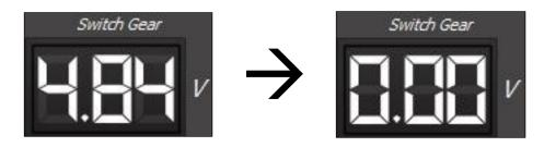
If voltage on the display **Switch Gear** doesn't switch down to 0 volt check the connections and modify the preload setting as described in **section 6**.
