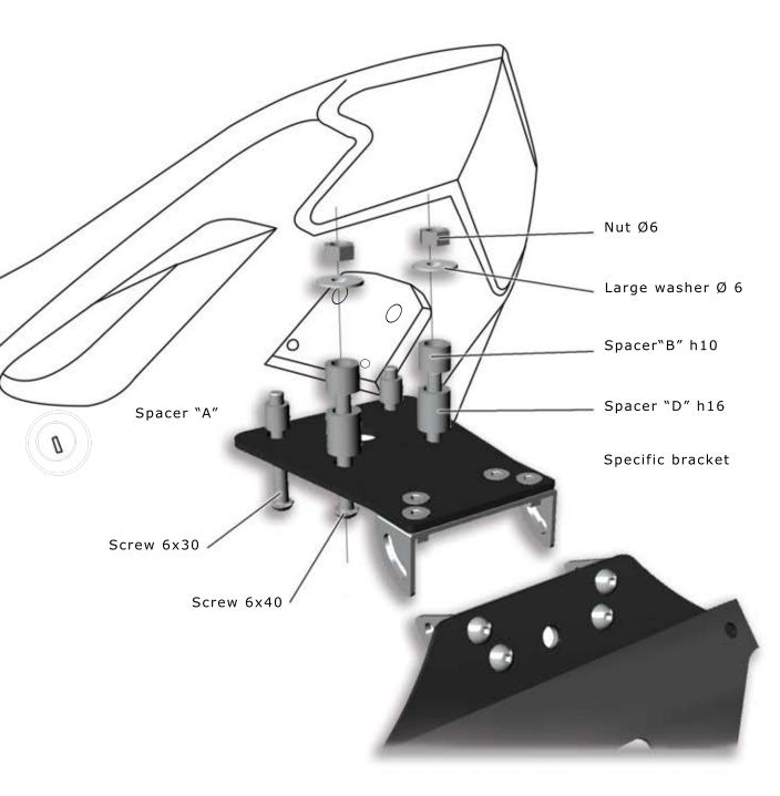
REMOVE THE ORIGINAL LICENCE PLATE. FIX THE BARACUDA SPECIFIC BRACKET USING THE THICKNESS AND SCREWS INCLUDED LIKE SHOWN IN THE PICTURE. REMOUNTING THE NUTS UNISTALL BEFORE TO LOCK THE SPECIFIC BRACKET OF LICENCE PLATE.
