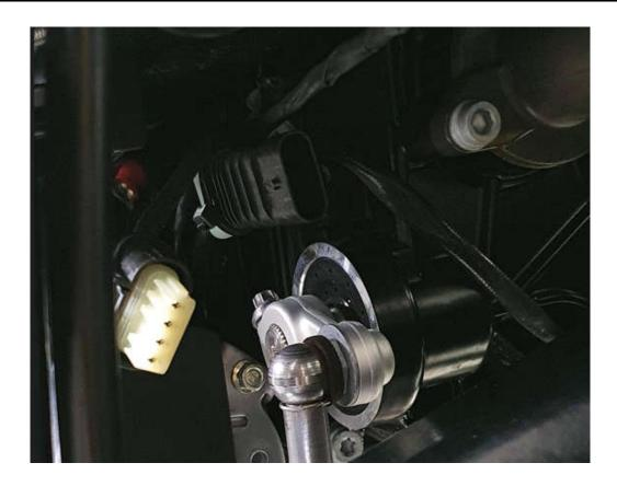
**8.2** Plug the connectors marked as **LN1** in-line with the stock wiring.
