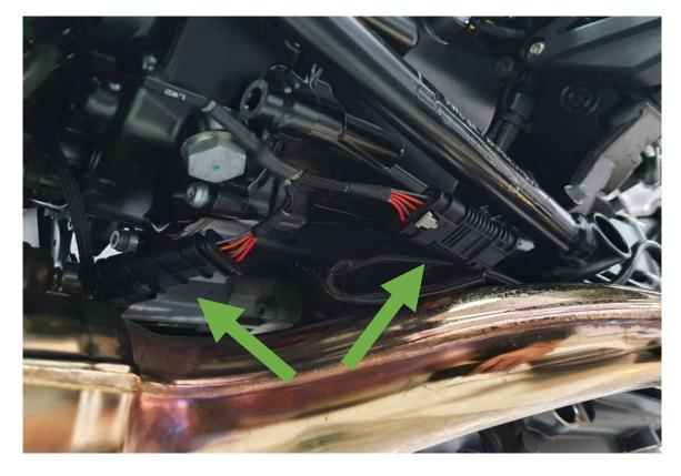
**6.4** Fasten all cables to the frame using zip ties.
