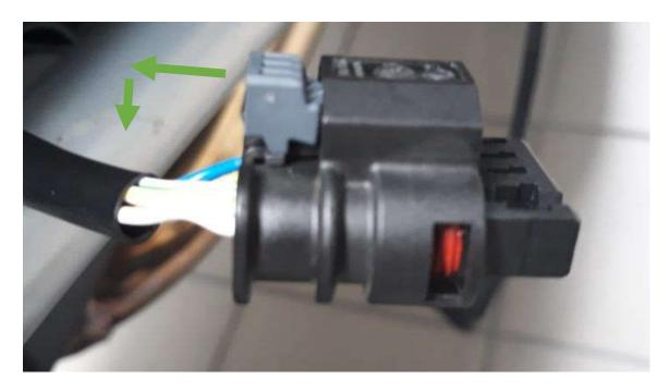
**6.3** Plug the connectors marked as **LW2** in-line with the stock wiring
