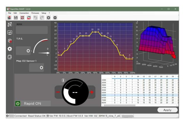
To connect with the SMART control unit, you only need an internal or external Bluetooth adapter to the PC at least release **4.0 BLE**. More information on the "Rapid Bike SMART" software manual, available with its installation.
