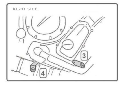
FIX THE ABS ENGINE SPOILER WITH ITS SCREWS KIT 4X10, WASHERS AND NUTS.
