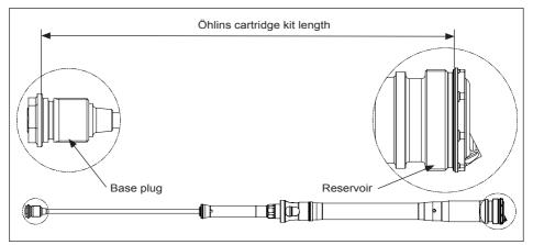
\*\*\*Measured to the bottom of the HEX 24 hydraulic stop cup
