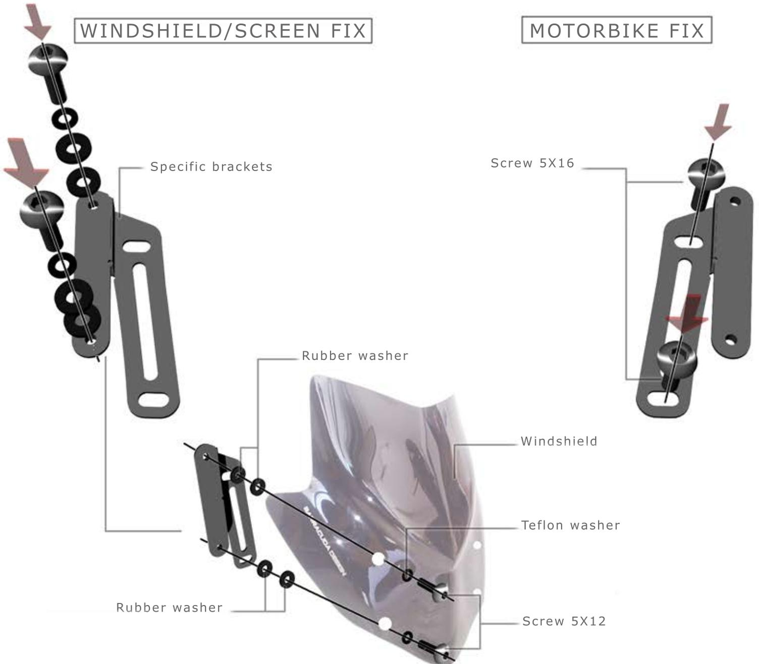
REMOVE THE ORIGINAL WINDSHIELD/SCREEN UNLOCKING THE 4 FIXING SCREWS, MOUNT THE SPECIFIC BRACKET WITH THE SCREWS LIKE DESCRIBED UP WITHOUT LOCKING TOO MUCH THE SCREWS, MOUNT THE WINDSHIELD/SCREEN ON THE BRACKETS USING THE RUBBER WASHERS, PUT THE WINDSHIELD/SCREEN IN THE CENTER MOVING INTO ALL DIRECTIONS, REMOVE THE WINDSHIELD/SCREEN AND LOCK THE POSITION OF THE BRACKET. MOUNT THE WINDSHIELD/SCREEN. DON'T LOCK TOO MUCH TO AVOID PLEXIGLASS DAMAGES
