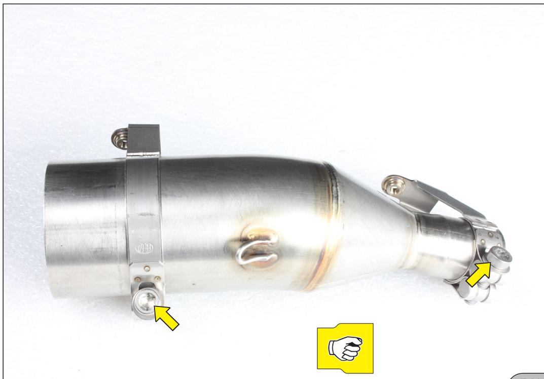
4. Assemble the link pipe with muffler and attach the springs (F 03, 04).
