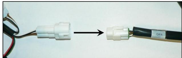
*If one or more My Tuning Bike are already installed, remove the **F27TERM1** and **F27TERM2** before installing Up/Down Shift Assist as they are not needed anymore.*
