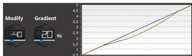
On software' screen, blue line indicates original proportion (1:1) between actual twist grip signal and signal received by OEM ECU, orange line shows new proportion and changes according to settings.
