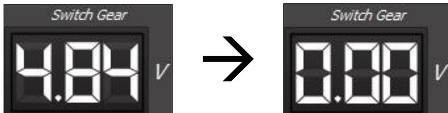
If voltage on the display **Switch Gear** doesn't switch down to 0 volt check the connections and modify the preload setting as described in **section 6**.
