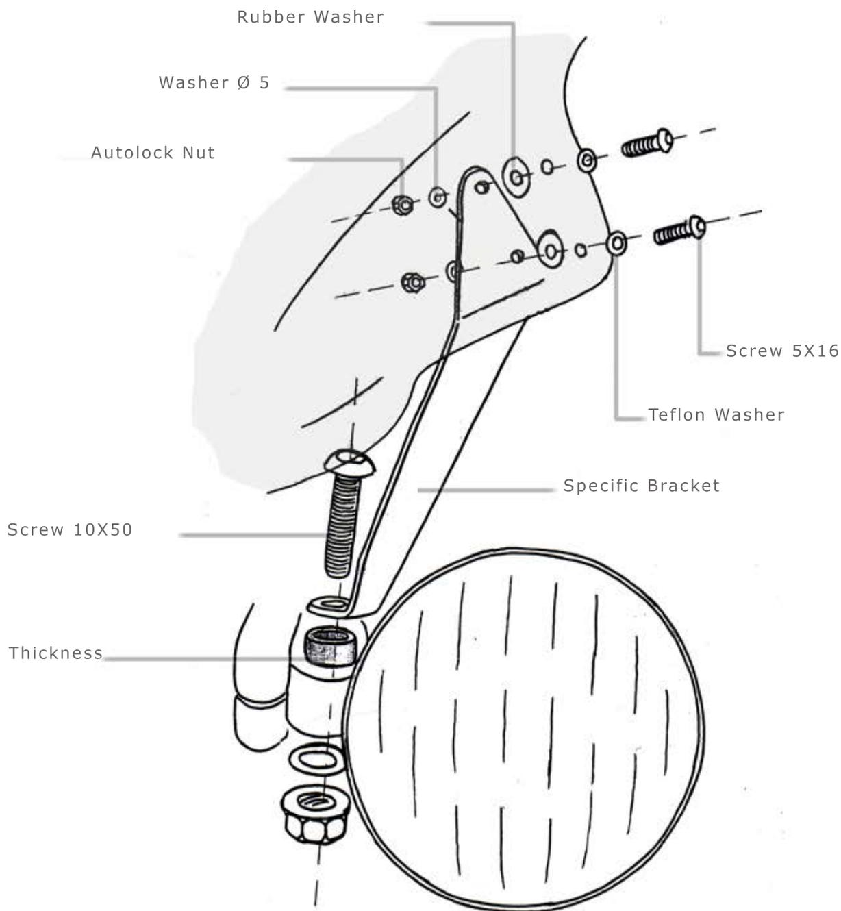
MOUNT THE WINDSHIELD/SCREEN LIKE DESCRIBED IN THE PICTURE UP. APPLY THE STICKER SQUARE RUBBER INSIDE OF WINDSHIELD/SCREEN TO AVOID CONTACTS WITH THE INSTRUMENTATION
