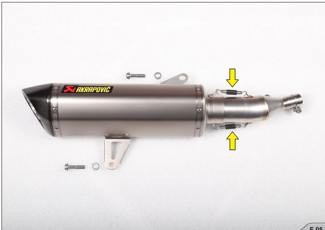
2. Carefully slide the muffler with link pipe onto the outlet side of the stock header pipe. Rotate the link pipe inside the muffler's inlet, until the muffler's brackets align with the two stock threaded muffler's brackets. Tighten the muffler bracket bolts (use washers and bolts from Akrapovič installation kit) and lambda sensor to the specified torques (**F 06**).
