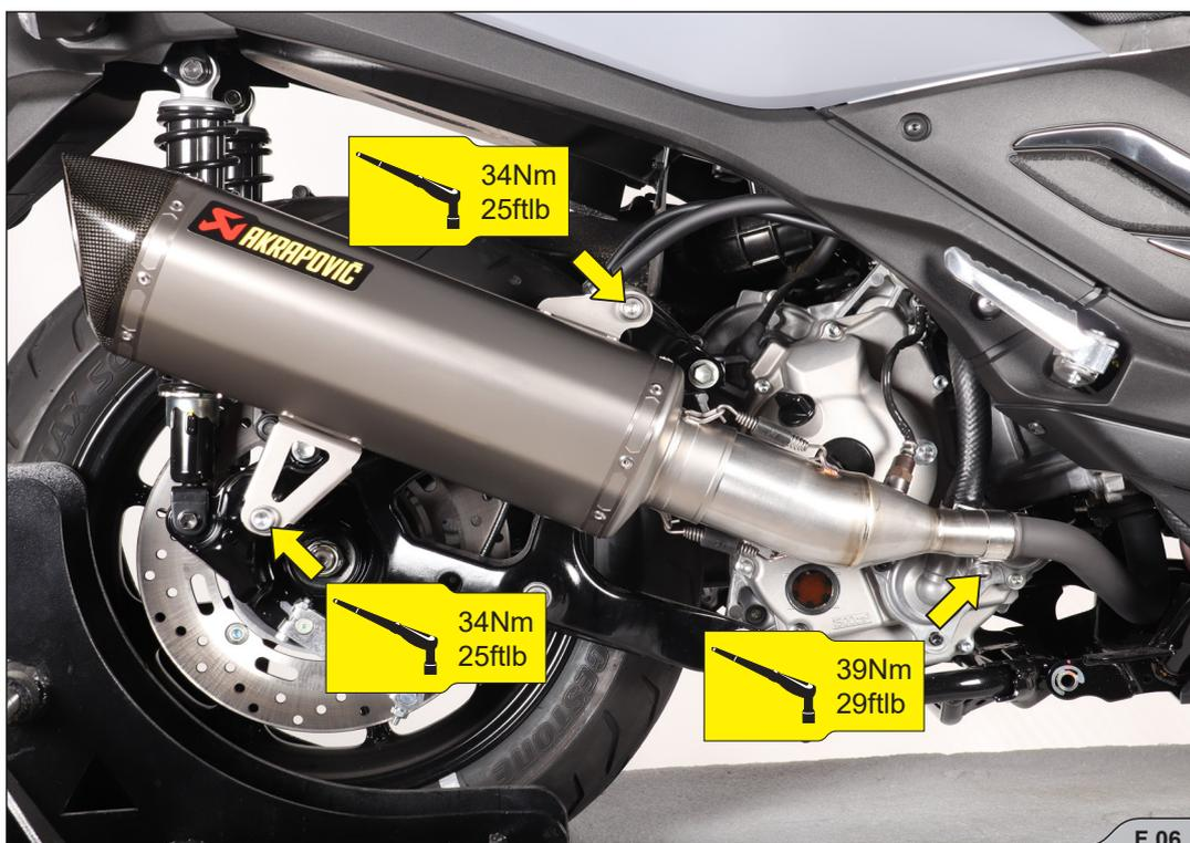
3. Tighten the marked clamp to the specified torque (F 07).
