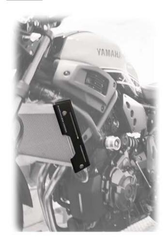
UNLOCK THE ORIGINAL FIXING POINT AND REMOVE THE ORIGINAL SIDE COVER.
