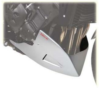
FIX THE ABS ENGINE SPOILER WITH ITS SCREWS KIT 4X10, WASHERS AND NUTS. APPROACH THE ENGINE SPOILER TO THE MOTORBIKE TO FIND THE FIXING POINT; MOUNT THE SPECIFIC BRACKETS USING THE ORIGINAL SCREWS OF CARTER WITHOUT LOCKING (SEE THE PICTURES); MOUNT THE ENGINE SPOILER ON THE BRACKETS USING THE 5X16 SCREWS AND THE RUBBER WASHERS BETWEEN THE ENGINE SPOILER AND THE BRACKET.
