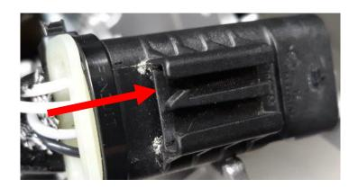
14. Plug the connectors marked as **LN1** in-line with the stock wiring.
