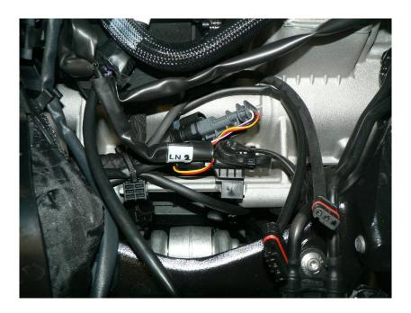
17. Ensure the wiring harness is properly fastened, then re-install fuel tank, side fairings and seats.
