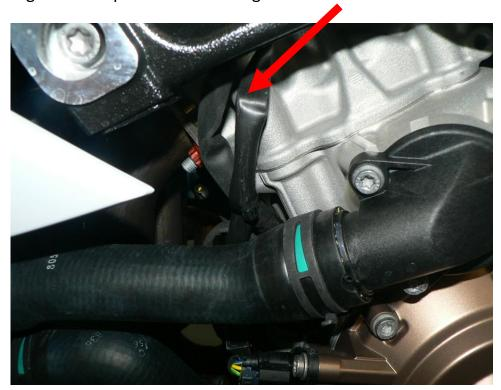
7. Fasten Rapid Bike wiring harness to OEM Lambda wiring harness using zip ties.
