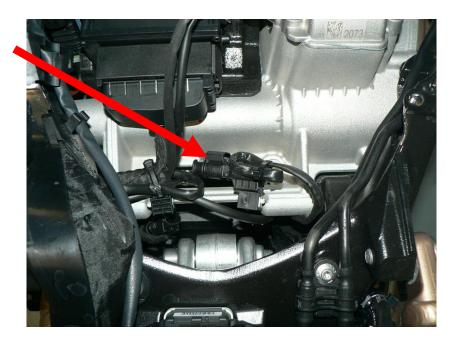
16. Plug the connectors marked as **LN2** in-line with the stock wiring.
